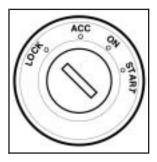
The ignition switch can be turned to four different positions with the key.
